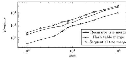
Figure 2.13: Recursive Trie Merge vs. Sequential Construction
