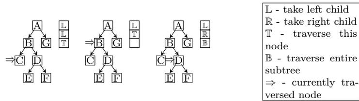
Figure 5.21: TreeIterator State Diagram
